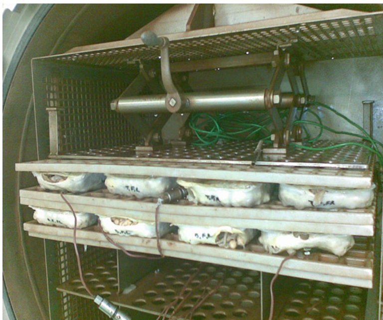
Fig. 11.1 Flexible retortable trays having burst as a result of insufficient overriding retort pressure during pilot plant retort experiment
