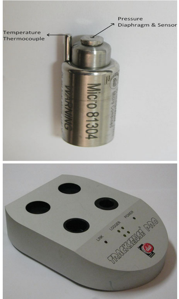
Fig. 11.3 Wireless instrumentation for measuring temperature and pressure, showing data logger (top) and logger reading station for downloading data files (bottom)
